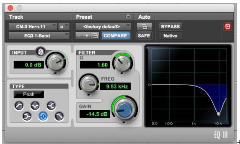
Figure 14. Single-band EQ applied to the French horn track to remove the cymbal high-end. 79
