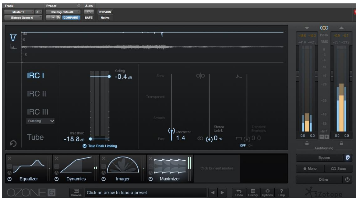
Figure 21. The maximizer in iZotope Ozone 6. The top blue line shows how the level going over the ceiling level and the meters on the right side illustrate how much of a volume boost the maximizer provided to the songs. 90
