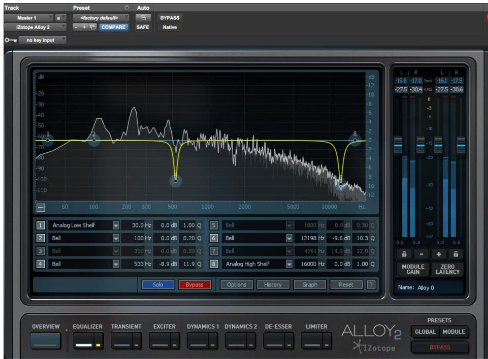
Figure 18. iZotope Alloy 2 equalizer plug-in used on the Master fader to notch out harsh frequencies in the room for the SPU Wind Ensemble Recordings. 87
