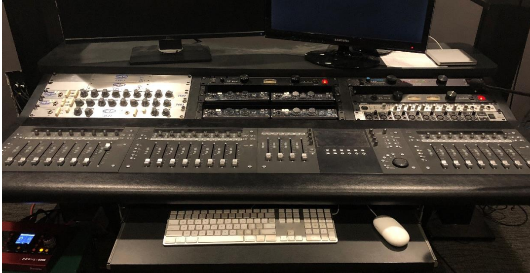
Figure 8. Nickerson Studios' mixing desk and preamps. The Chameleon Labs preamps are light gray and located on the left, Grace Design preamps are in the middle, and Mackie preamps are on the right. The RedNet preamps are in the patch bay rack. 71
