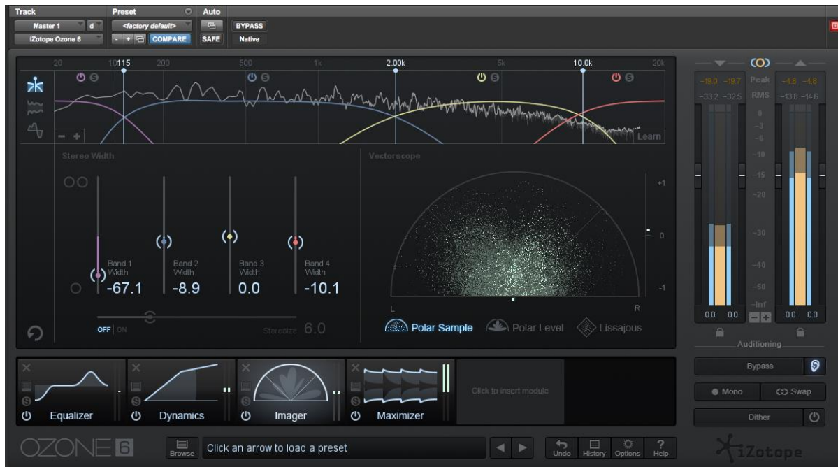
Figure 20. Imager in iZotope Ozone 6 which shows the frequency spectrum and polar sample of the song at the time the screenshot was taken. 89
