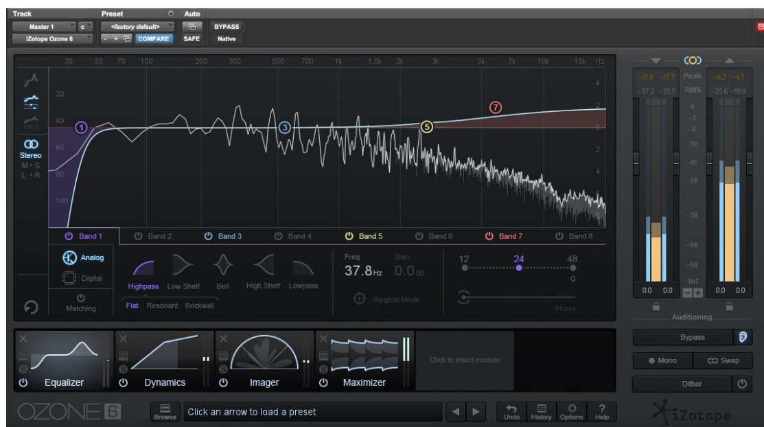
Figure 19. Equalizer in iZotope Ozone 6 showcasing an HPF and high frequency shelf. 88
