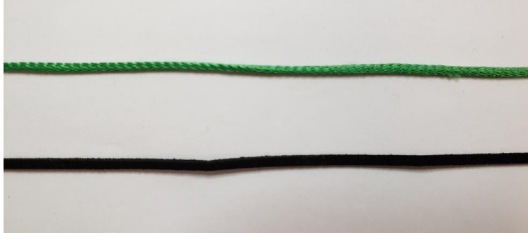
Figure 4: Image of Two Cords Tested Green Sting (Top) and Sueded Cord (Bottom)
