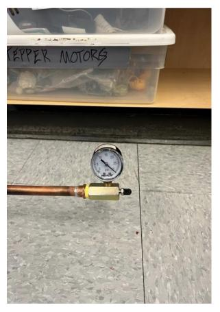
We left the pressure test for the panel plumbing for about a week and experienced no leaks.
